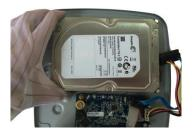
3. Match the screws with the holes on the DVR to place the HDD.
