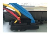
5. Use the HDD cable and power cable to connect HDD and mainboard.
