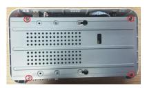
Install the bracket back and then fasten the screws.
