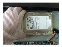
3. Place the HDD onto the Device.
