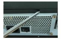
Loose the screws on the panel and remove the cover.
