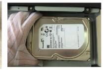
Put the HDD into the Device.
